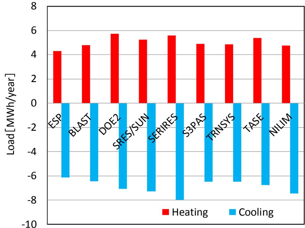
Simulated Heating and cooling loads
