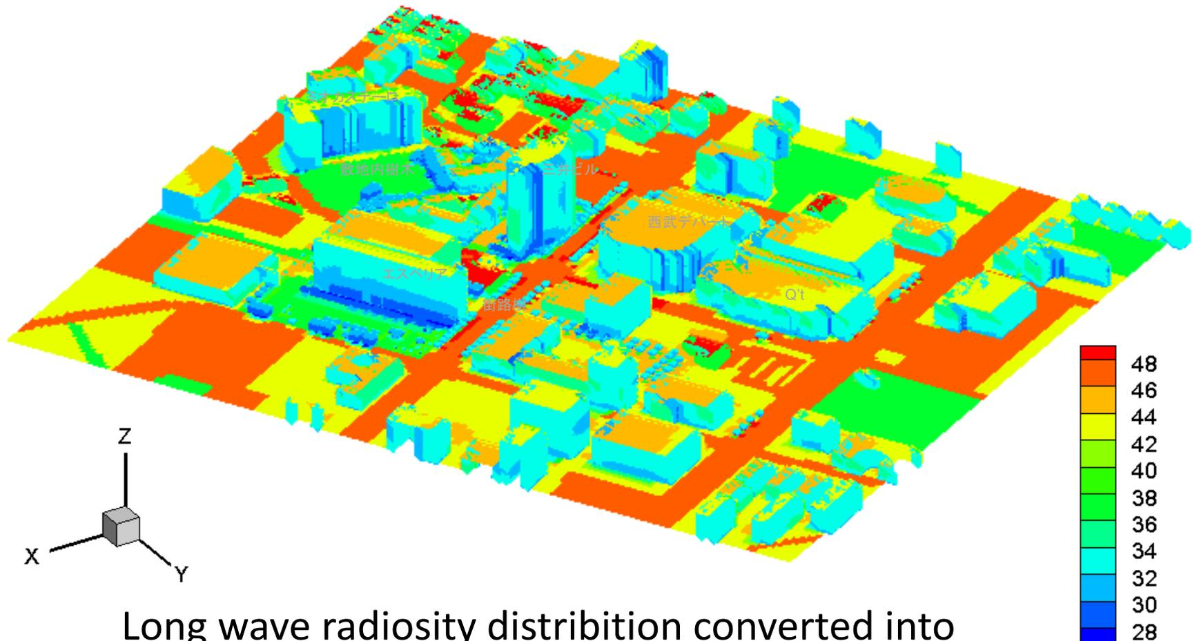
Long wave radiosity distribution converted into surface temperature distribution
