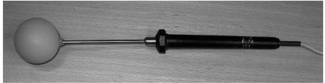
Figure 3. The 38 mm flat grey globe thermometer.
