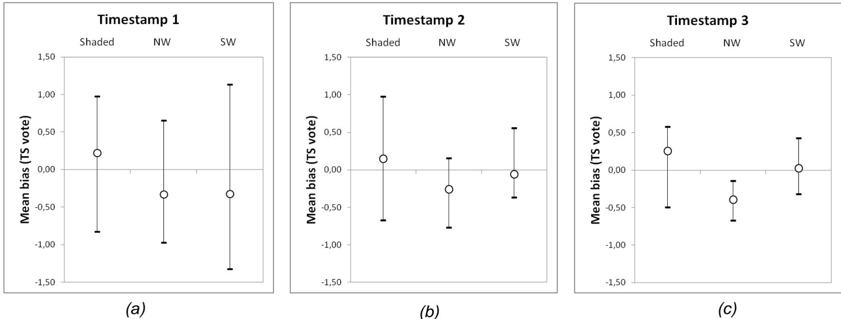
*Mean bias (DTS-TSV) with minimum and maximum bias as error bars for the three window configurations, a) immediately after leaving the chamber @ timestamp 1; b) after 15 minutes @ timestamp 2; c) after 30 minutes @ timestamp 3*
