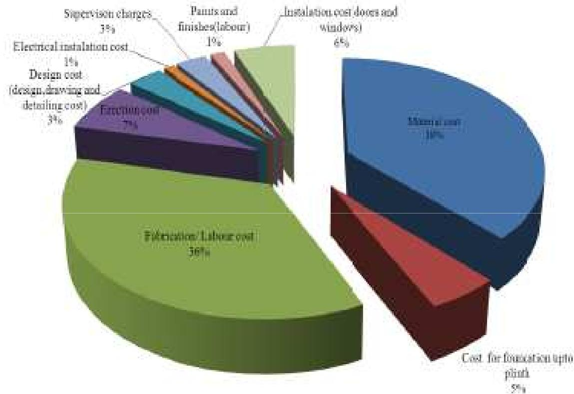
Fig.8.11 Cost estimates for 45 sqm experimental demonstration structure under R & D mode;
