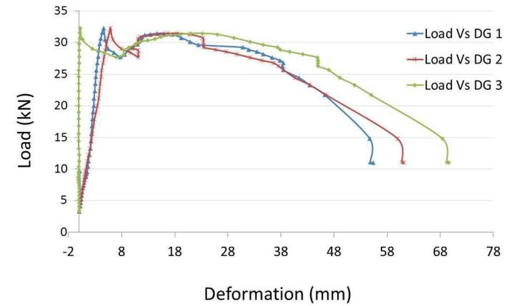
Failure of Concrete Band at 33 kN Load
