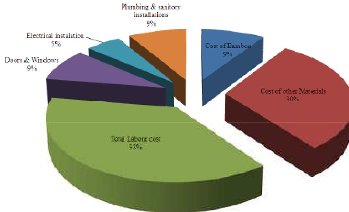
Fig. 8.12 Cost estimates for 27 sqm structure under replication mode; Total Cost of Structure = Rs. 1.17 lakhs; Total Area of Construction = 27 m<sup>2</sup>; Cost per Sq m. = 4276; Cost per Sqft = Rs. 385 per sq. ft. & Estimated time = 10 days with a team of 18 artisans
