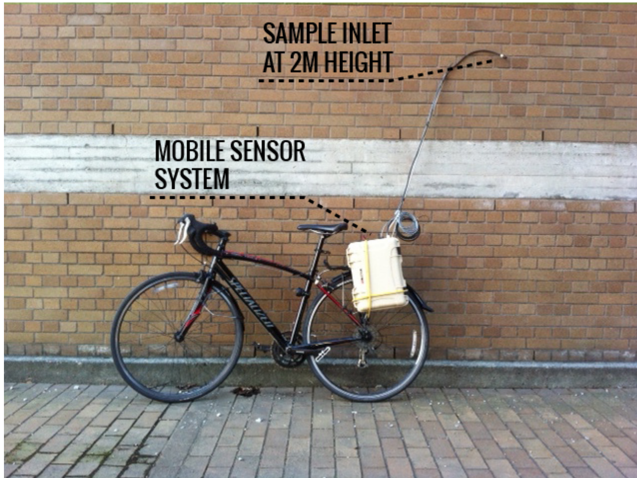
Image: Shows the installation of the sensor on a bike rack – the inlet is at approximately 2m height.
