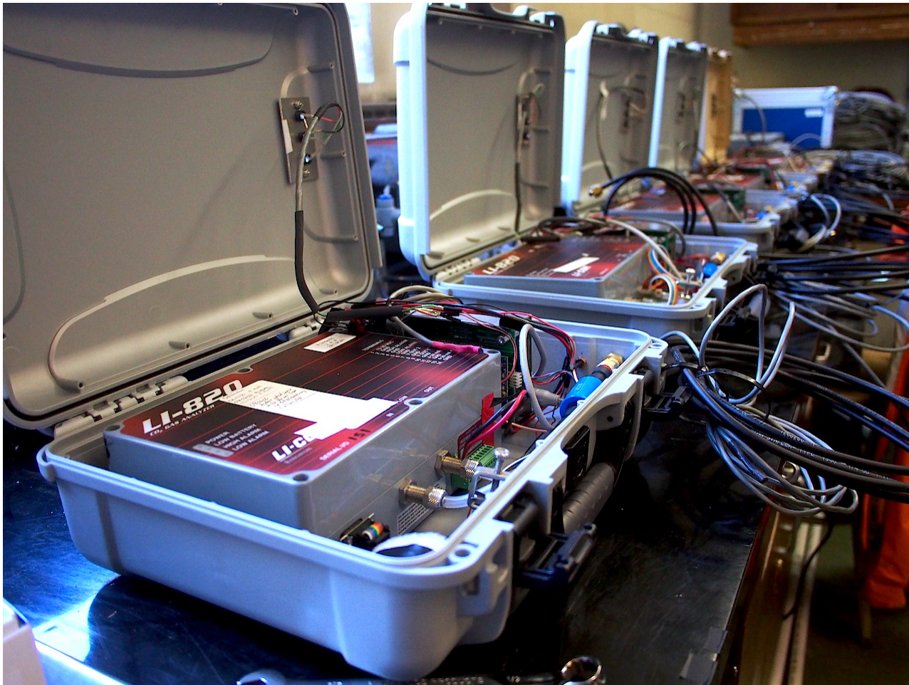
Image: In total 5 sensors were built – the image shows the full setup including the sample inlet tube and the temperature probes.
