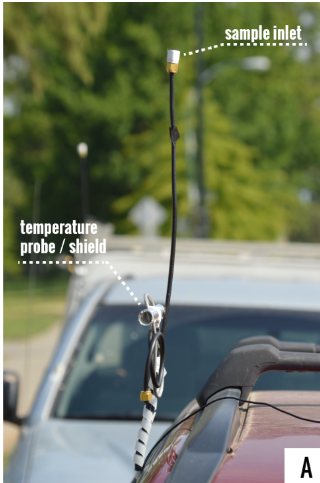
Image A: Shows the temperature probe covered by PVC tube and reflective tape and sample inlet tube at 2m height - \pm 0.5^{\circ}\text{C} Accuracy from -10^{\circ}\text{C} to +85^{\circ}\text{C} ; Image B: Shows sensor installation in vehicle.
