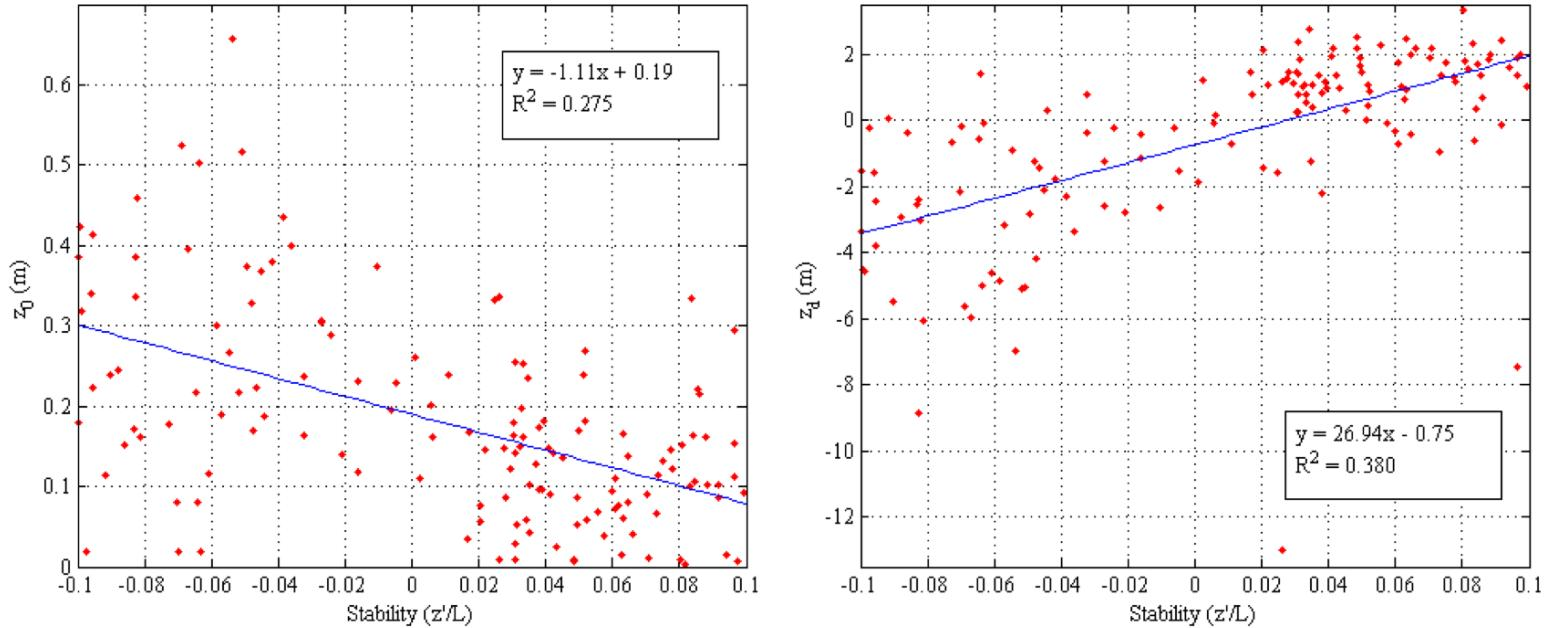
Figure 6: Estimated surface roughness length ( $z_0$ ), left, and zero-plane displacement height ( $z_d$ ), right, plotted as functions of the dimensionless stability parameter ( $z'/L$ ) for all Sector V Event Week observation periods.
