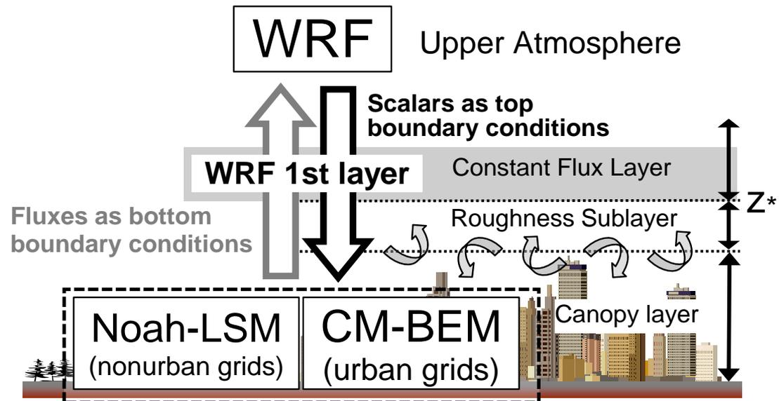
Two-way coupling of CM-BEM with WRF
